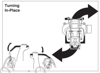
Figure 7. Turning in Place
